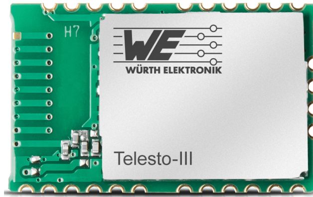
Figure 5: Telesto-III: proprietary 915 MHz radio module
