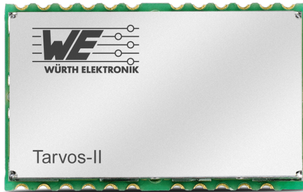
Figure 7: Tarvos-II: proprietary 868 MHz radio module
