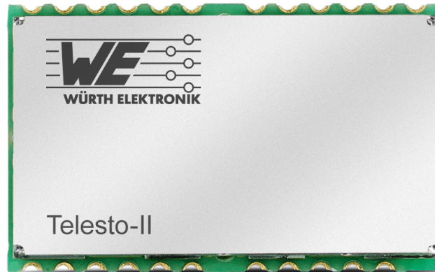
Figure 10: Telesto-II: proprietary 915 MHz radio module
